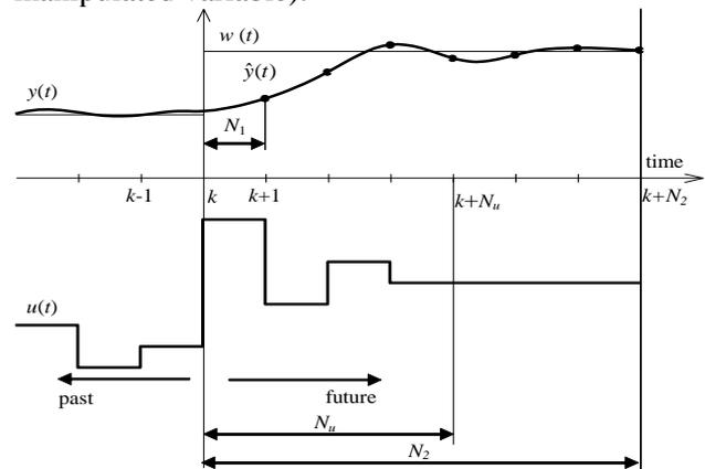
Fig. 1 Principle of predictive control
