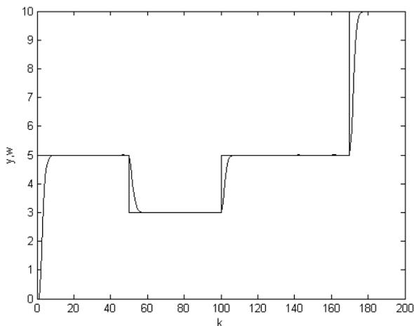
Fig. 3 Controller based on polynomial methods-control without disturbance
