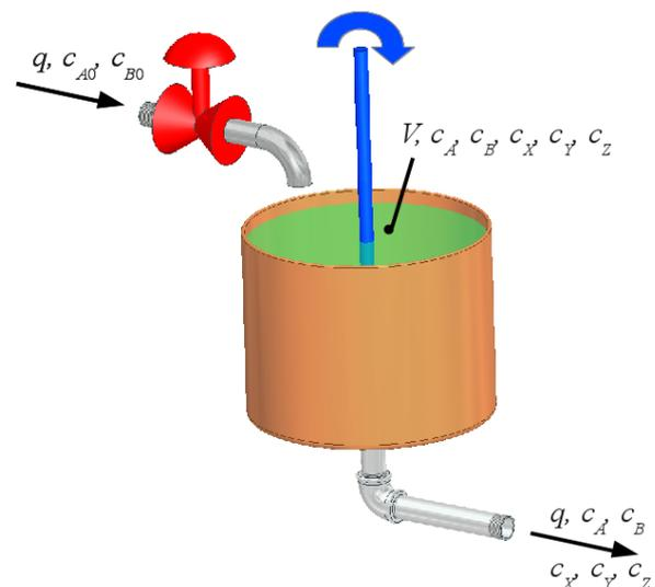
Fig. 1 Scheme of the isothermic Continuous Stirred Tank Reactor
