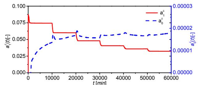
Fig. 13 The course of the identified parameters  $a_1^\delta$  and  $a_0^\delta$  for control with Pole-placement method
