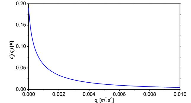
Fig. 5 The steady-state characteristics of concentrations  $c_Z$  for various volumetric flow rate  $q$
