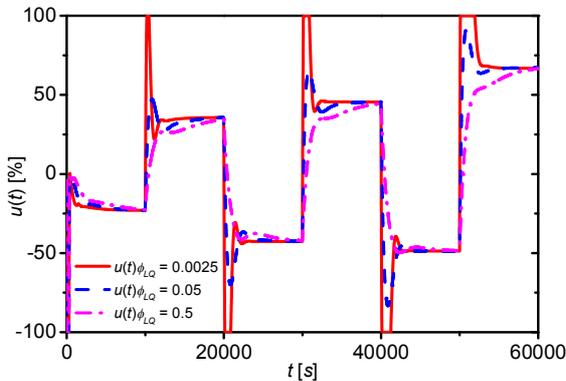
Fig. 16 The course of the input variable,  $u(t)$ , for the control with LQ method
