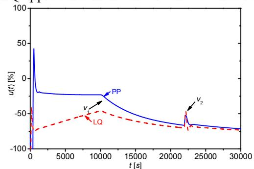
Fig. 20 The course of the input variable,  $u(t)$ , for pole-placement (PP) and LQ approaches in the disturbance attenuation
