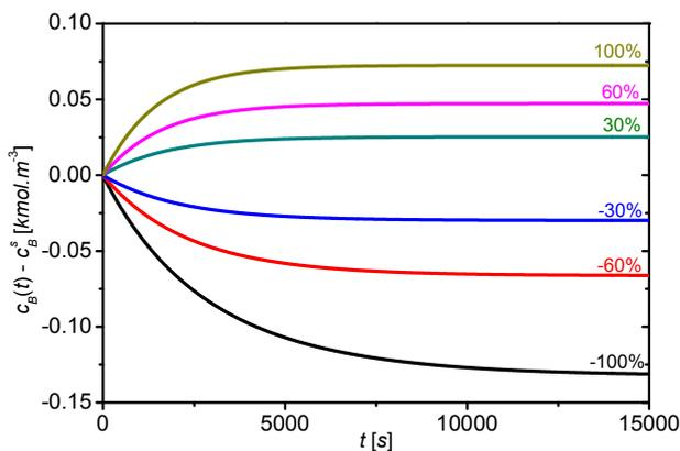
Fig. 6 The dynamic characteristics of the concentration  $c_B$  after step changes of input volumetric flow rate  $q$
