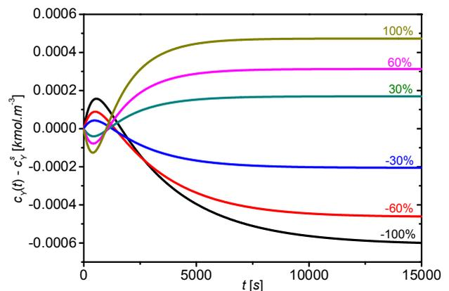
Fig. 8 The dynamic characteristics of the concentration  $c_Y$  after step changes of input volumetric flow rate  $q$
