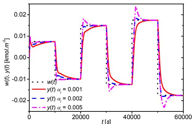
Fig. 11 The course of the output variable,  $y(t)$ , and the reference signal,  $w(t)$ , for the control with Pole-placement method
