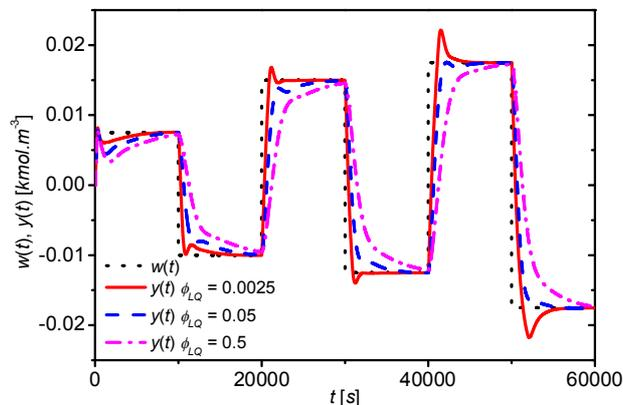
Fig. 15 The course of the output variable,  $y(t)$ , and the reference signal,  $w(t)$ , for the control with LQ method
