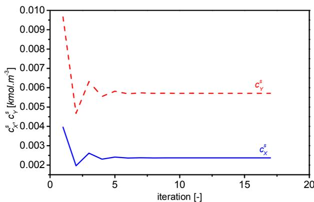
Fig. 2 Computation of the steady-state values of concentrations  $c_X$  and  $c_Y$  through the iterations
