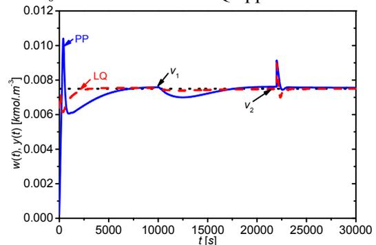
Fig. 19 The course of the output variable,  $y(t)$ , and the reference signal,  $w(t)$ , for pole-placement (PP) and LQ approaches in the disturbance attenuation
