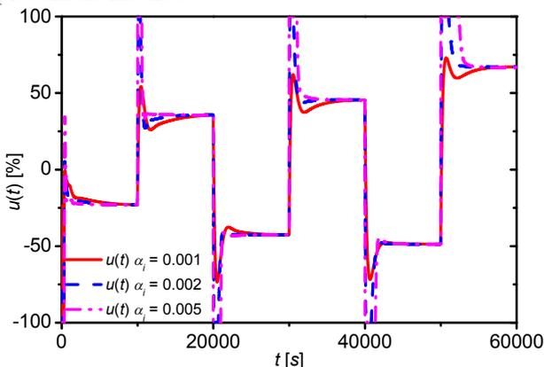
Fig. 12 The course of the input variable,  $u(t)$ , for the control with Pole-placement method
