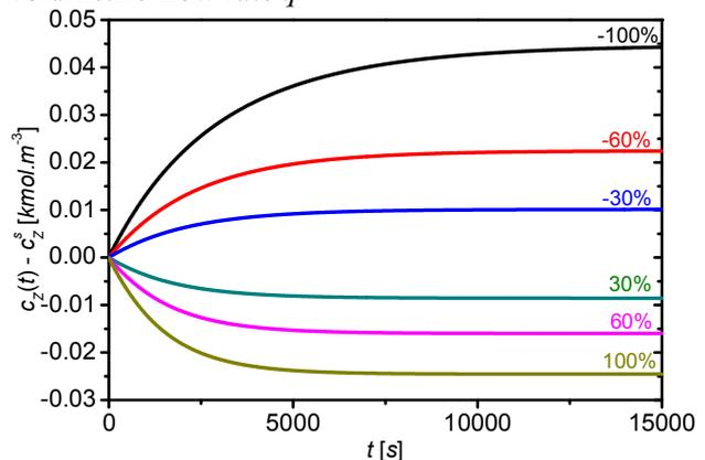
Fig. 9 The dynamic characteristics of the concentration  $c_Z$  after step changes of input volumetric flow rate  $q$
