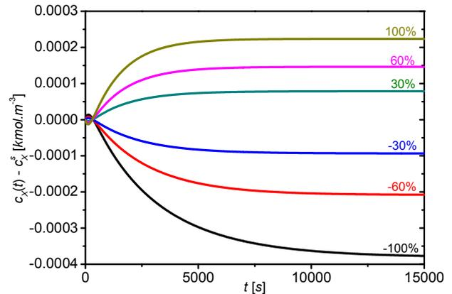
Fig. 7 The dynamic characteristics of the concentration  $c_X$  after step changes of input volumetric flow rate  $q$
