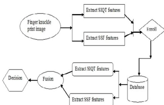
**Fig. 3. Architecture diagram of the proposed FKP based system for recognition**
