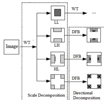
Figure 2 Decomposition of WBCT (First Level)
