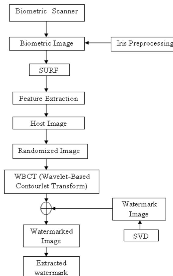
Figure 1 Overall Process of the Proposed System
