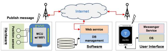
Fig. 1 Architecture of hardware, software and user interface
