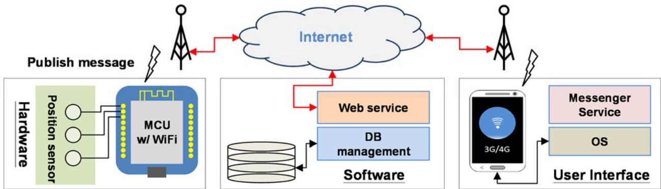
Fig. 1 Architecture of hardware, software and user interface
