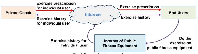
Fig. 3 Proposed system procedure
