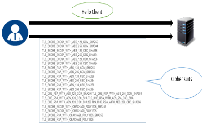
Fig. 5. Starting an SSL Negotiation
