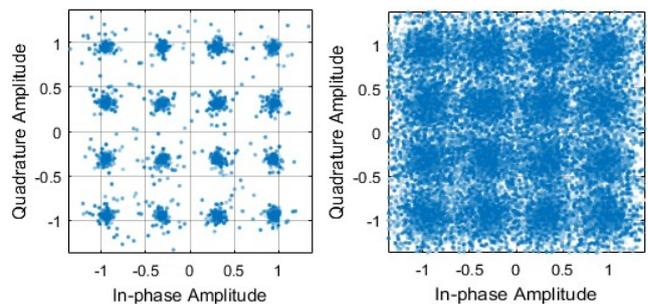
Fig. 8: Receiver constellation with SNR=36(dB) and 14(dB)
