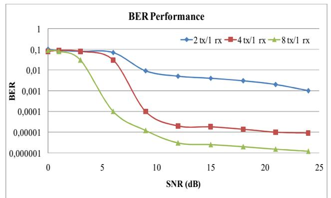
Fig. 7: BER performance of MIMO-OFDM 802.11ad system
