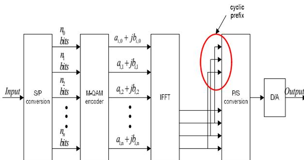
Fig. 3 OFDM transmitter
