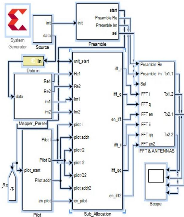
Fig. 5: MIMO-OFDM 802.11ad Transmitter implementation
