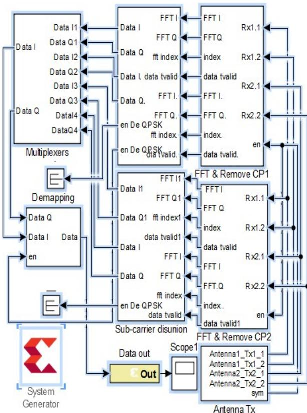
Fig. 6: MIMO-OFDM 802.11ad Receiver implementation
