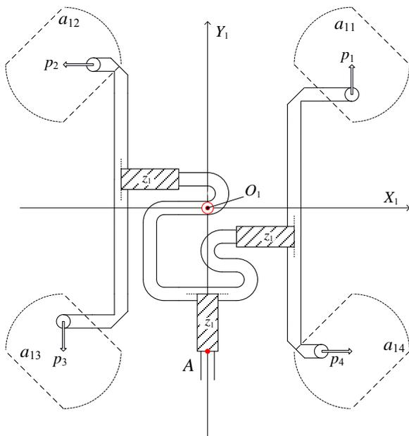
Fig. 3 Smoothed routing wire for a 4-antenna  $a_{11} \sim a_{14}$ , and  $p_1 \sim p_4$  are feeding Poynting vectors at the first quadrant.  $O$  is the centre of the plane  $X_1 - Y_1$ .  $A$  is the input point of feeding.  $z_1$  and  $z_0$  are characteristics impedances of routing wires.
