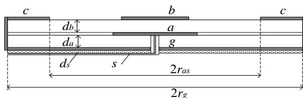
Fig.1 Cross sectional view of the proposed antenna.
