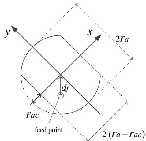
Fig. 2 Main element  $a$  with feeding.
