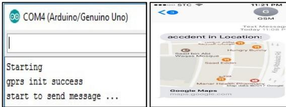
Fig. 12. (a) GSM Sending SMS(b) Received SMS Location by the mobile
