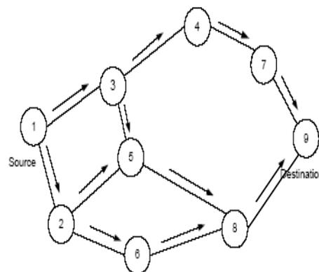
Fig. 3. The Route Request packets flooding in AODV
