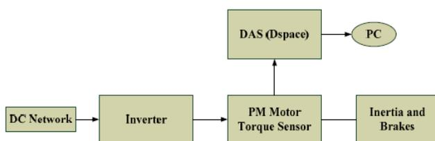
Fig. 3 Testing bench for motor measurements
