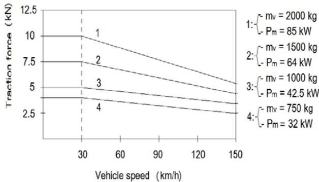
Fig. 1 Traction characteristics.
