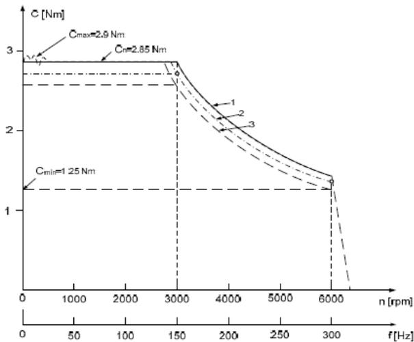
Fig. 5 Experimental torque curves of PM motor
