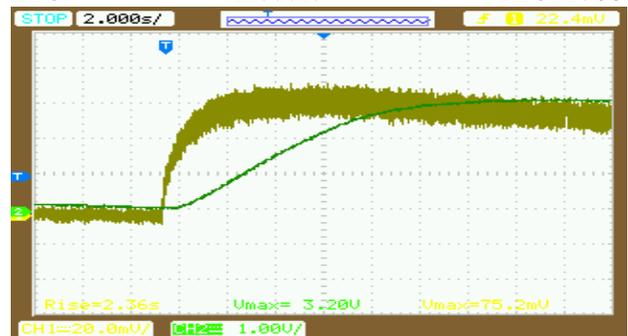
Fig. 7 the output voltage sequencing with 47kΩ load
