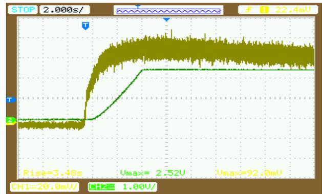
Fig. 10 output sequencing with white LED load
