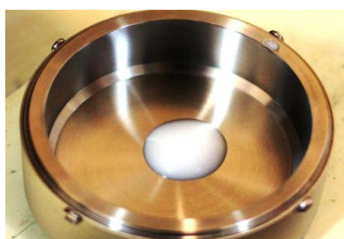
Fig. 3. A sample of cooled polidocanol foam in viscometer cell before measurement
