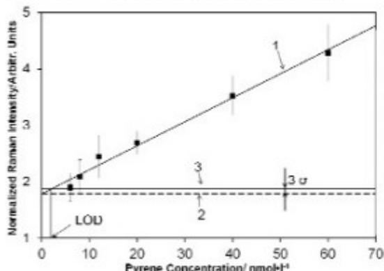
Figure 1: Standard approach for LOD calculation. The Raman band of pyrene at  $1239\text{ cm}^{-1}$  was used for creating the calibration curve at low concentrations up to  $60\text{ nmol/L}$  (solid line 1). The dashed (2), long dashed-dotted (3) and vertical solid (4) lines mark the mean blank signal, the blank signal standard deviation and the LOD projection, respectively.
