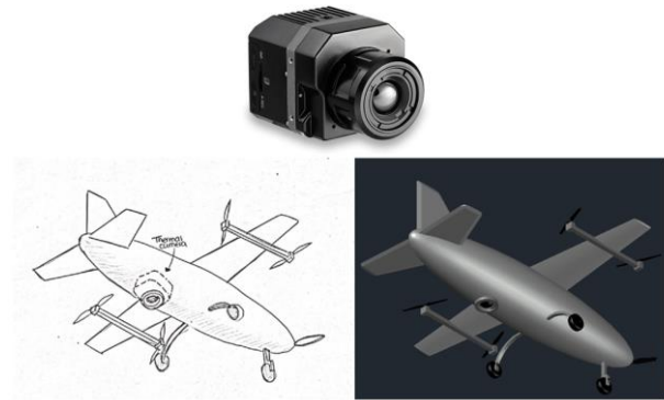
Figure 5: Thermal camera and its location
