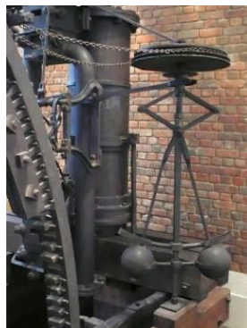
Fig. 3. Centrifugal governor in a Boulton and Watt engine of 1788
