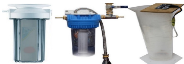
Fig.10. (a) Typical Bubbler (b) Multipurpose bubbler (c) Level tube to calculate amount of gas by ultrasonic sensor
