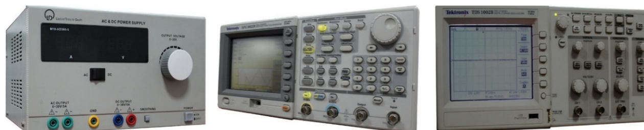
Fig. 5. (a) DC/AC Power Supply (b) Function Generator– Model AFG 3022B Tektronix (c) Digital Oscilloscope
