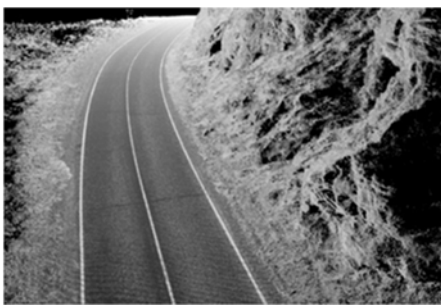
Fig.3. A resulting cloud of laser scanning points includes reflections from people, equipment, vegetation, etc. located on the object
