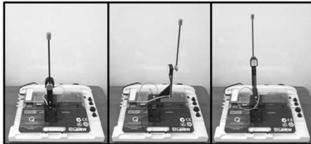
Figure 11: Sequence frame of the Furuta's pendulum for step change reference ( \theta = 0.872[rad] ) with FLC
