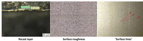
Fig. 1: Main surface defects during surfacing in WEDM
