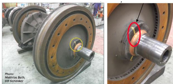
Fig. 1 locomotive wheelset with marked relative rotation (see yellow indication mark in the red ellipse on the right part of the picture) [1]
