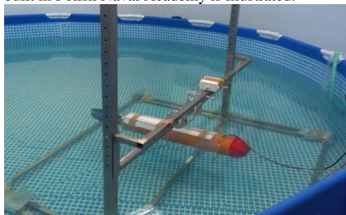
Fig. 5. The laboratory stand for measurement of the thrust generated by an underwater vehicle built in Polish Naval Academy [9]
