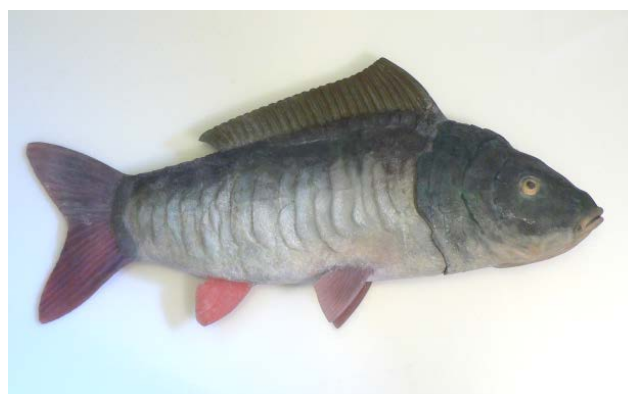
Fig. 2. BUV CyberFish ver. 5 in silicon coating [5]
