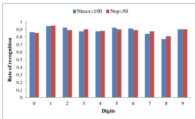
**Fig.7, Rates of recognition with optimal size 50 neurons and 100 neurons with 48 states**
