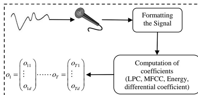
Fig.1, Acoustic analysis step
