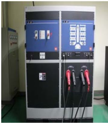
Fig. 14 The AV900 power system
