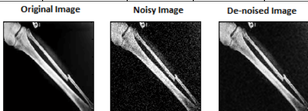
Figure 11: Denoising results of Dual Tree Complex Wavelet Transform for XRAY Image (Gaussian Noise – variance = 0.01) (a) Original (b)Noisy (PSNR=20.7678 dB) (c) Recovered (PSNR=27.4066dB)
