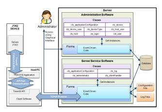
Fig. 12 Detailed View of the Server Service and Administration Software
