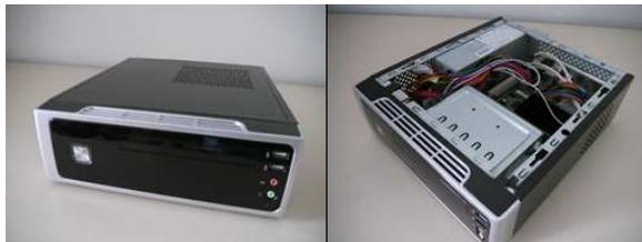
Fig. 8: Suitable HW platform containing x86 Intel Atom 1.6GHz, RAM 1GB/677MHz and 16GB SSD.
