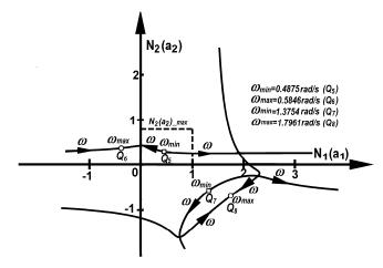
Fig.8. Root-loci Analyses of limit cycles of Example 1 for  $k_1 = k_2 = 1$ .
