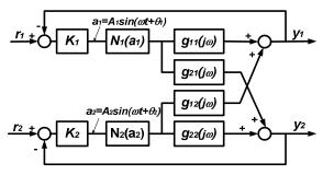
Fig.2. A 2x2 Nonlinear Multivariable Feedback Control System.
