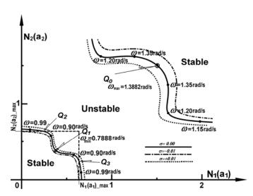
Fig.3. Root-Loci of limit cycles in the parameter plane.
