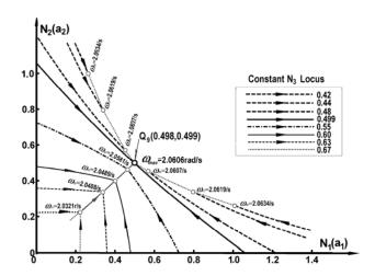
Fig.10. Root-loci analyses of limit cycles of Example 2 on  $N_1(a_1)$  vs.  $N_2(a_2)$  Plane for  $N_3(a_3)$  varying and  $k_i=1$ ..
