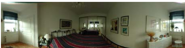
Fig. 10: Flattened 360-degree panoramic image obtained from a donut-shaped PAL image of Fig. 9
