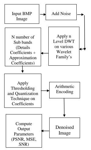
Fig.7 Proposed Block Diagram of image denoising using Wavelet Thresholding Technique
