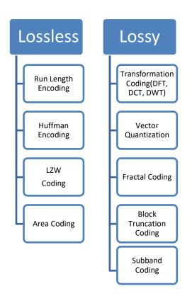
Fig.1 Types of Compression Algorithms in Medical Imaging
