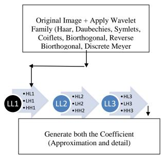
Fig.8 The process of generation of wavelet Coefficients
