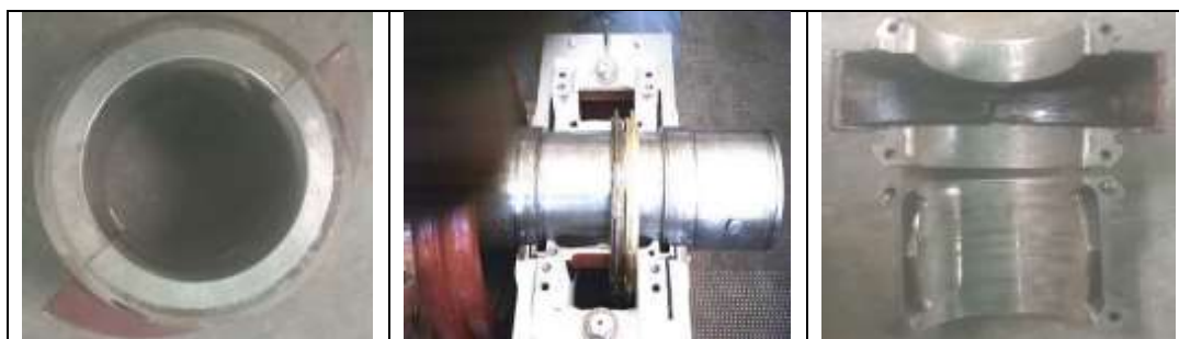
Fig. 1: Sleeve bearing lemon shape with two oil ring
