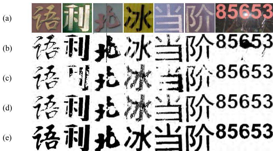
Fig.10 Examples of text binarization: (a) Original character images, (b) Binarization by color clustering in RGB space, (c) Binarization by color clustering in HSI space, (d) Initial binarization result, (e) Refined by Graph cut algorithm
