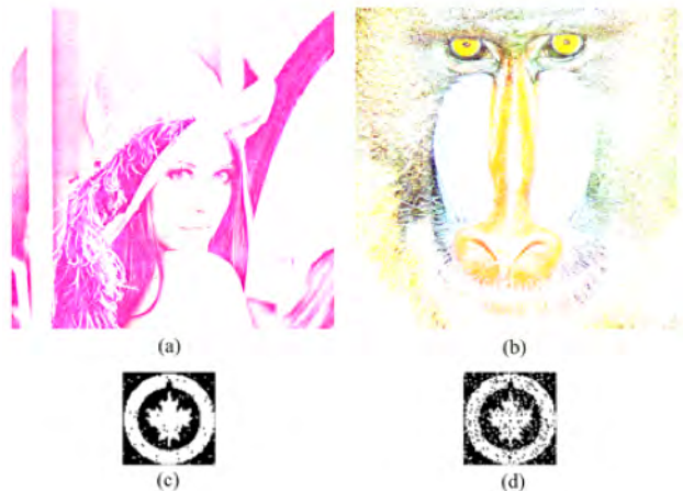
Figure 14: An example of amplitude scaling attack and watermark extraction with SF=0.3 : (a) scaling the watermarked image of Lena at Fig. 10(b) with SNR=-7.36 dB, (b) scaling the watermarked image of Baboom at Fig. 10(d) with SNR=-7.36 dB, (c) the extracted watermark from (a) with WAR=98.09 %, (d) the extracted watermark from (b) with WAR=90.09 %.
