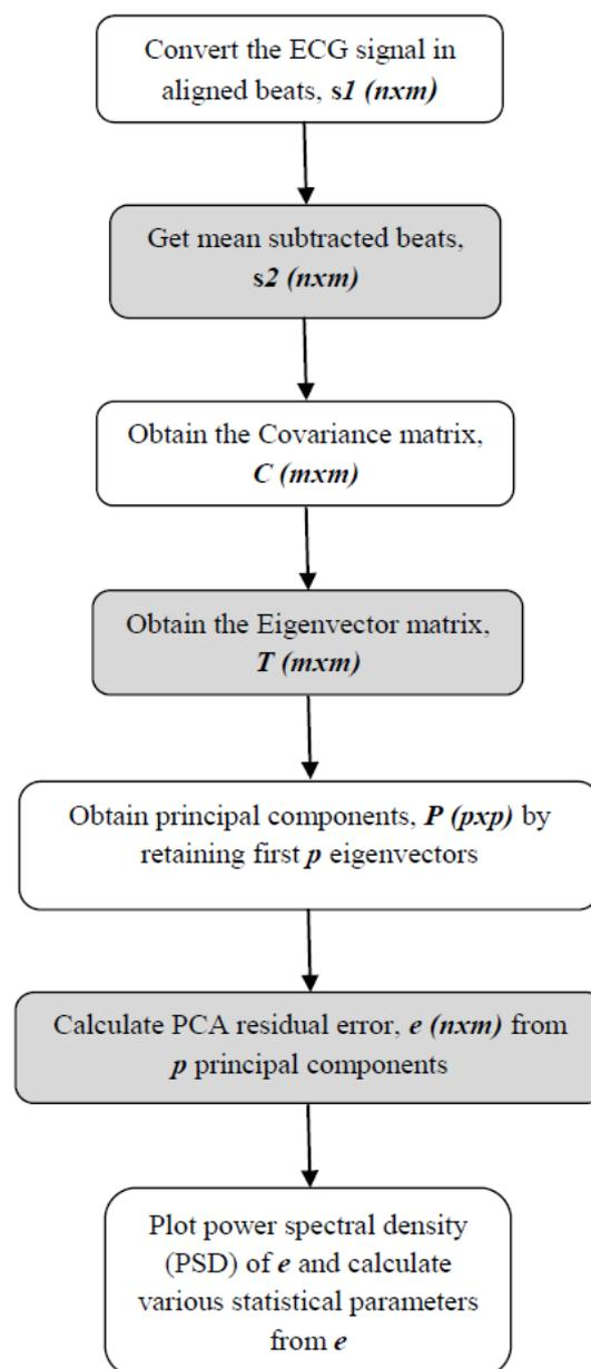
Fig. 4. PCA based algorithm for spectral characteristics of motion artifacts
