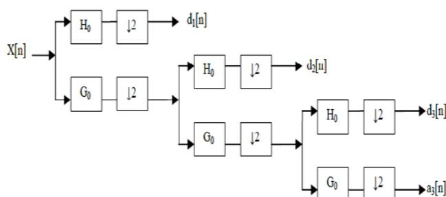
Fig. 5. A three-level Wavelet decomposition.
