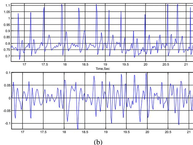
Fig. 6. (a) W-ECG signal recorded with Biopac MP-36 recorder (top) and extracted motion artifact signal (bottom); (b) similar results for W-ECG signal recorded with wearable recorder
