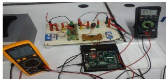
**Figure 23.** Hardware set-up for Boost converter for PV.
