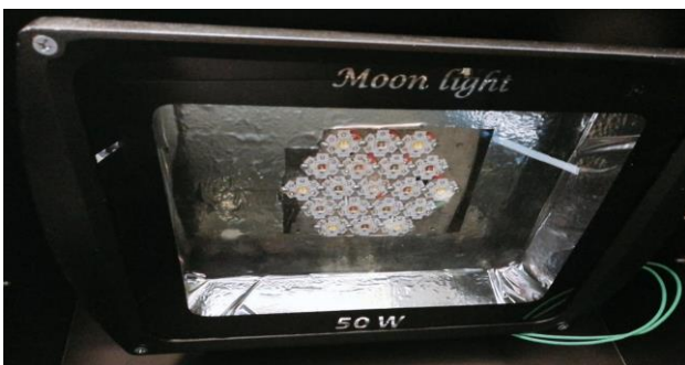
Fig.16: The distribution structure of LEDs for solar simulator
