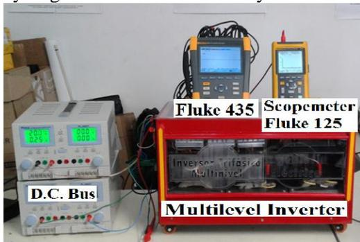
Fig. 6 Assembly of the test
