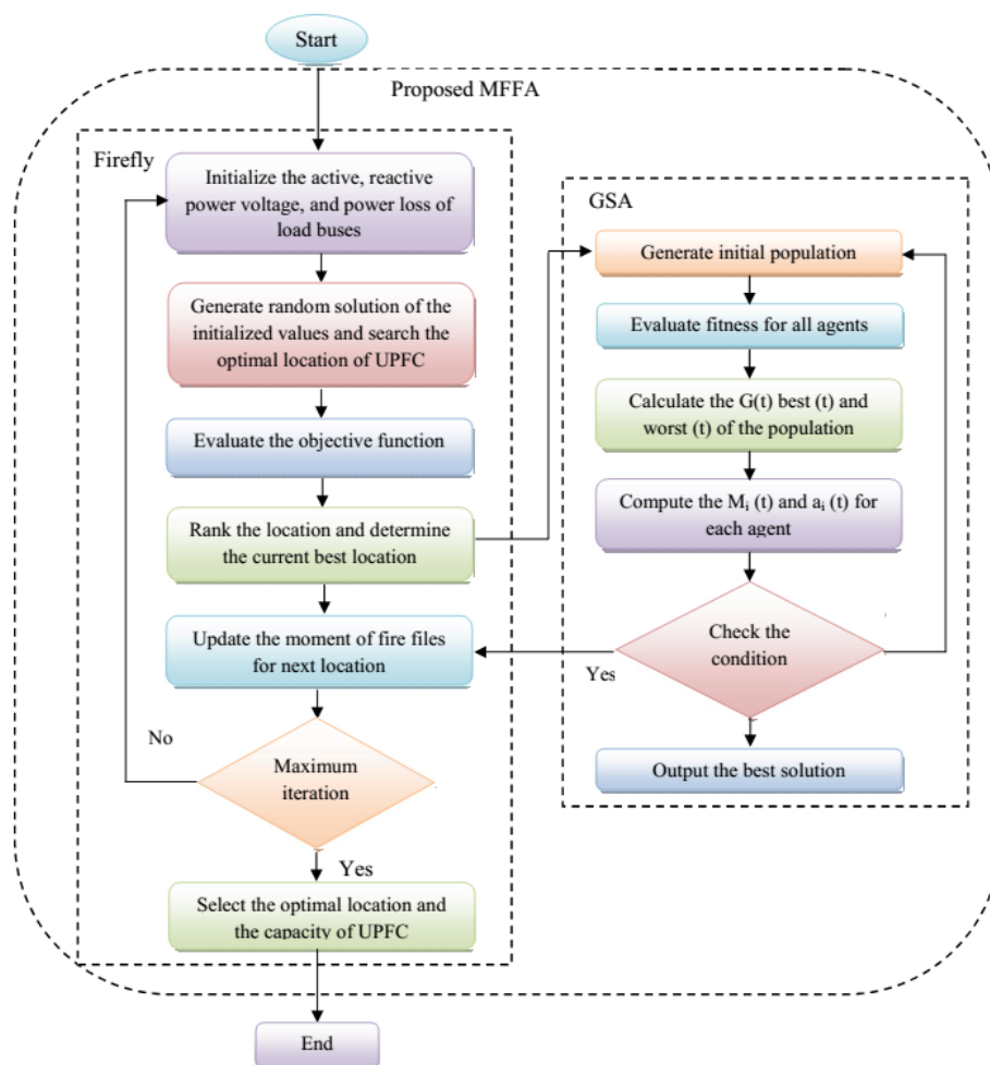
Figure.3: The flow chart for the proposed MFFA
