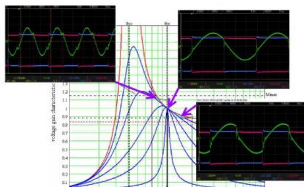
Fig. 13 Example of the interpretation of voltage gain characteristics and relevant operational waveforms of LLC converter during various conditions
