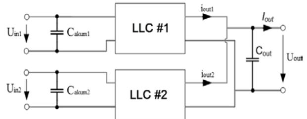
**Fig. 10** Principle of the separated input voltage for parallel connected LLC converters
