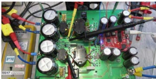
**Fig. 14** Experimental prototype of high power density dual interleaved LLC resonant converter
