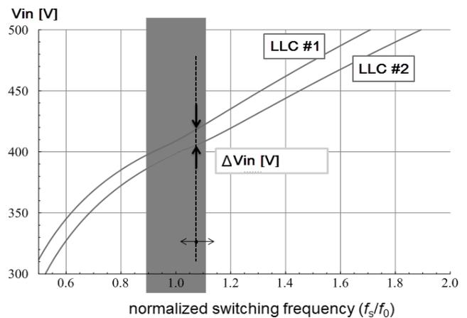
**Fig. 11** Impact of the tolerance of resonant components on resonant frequency deviation
