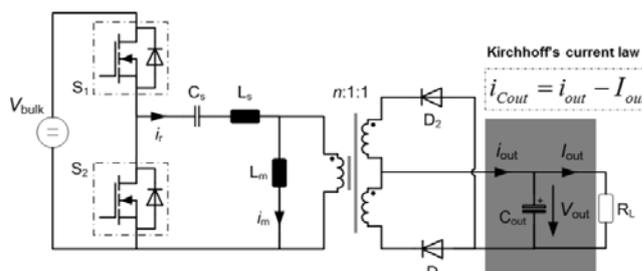
Fig. 7 Typical schematic of the LLC converter
