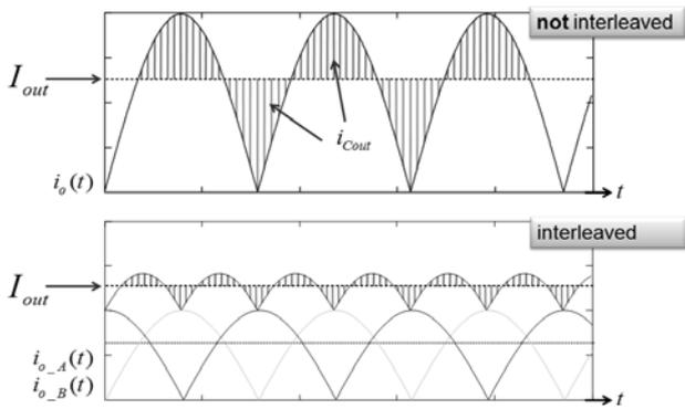
**Fig. 8** Influence of interleaving for reduction of output capacitor's ripple current
