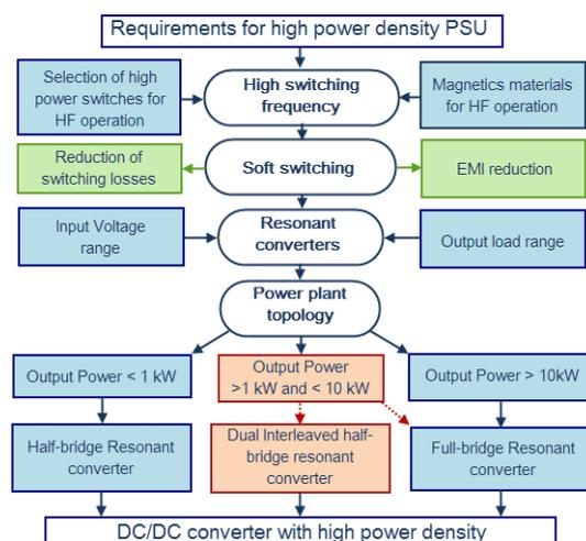
**Fig. 1.** Simplified design procedure for high power density DC/DC converter
