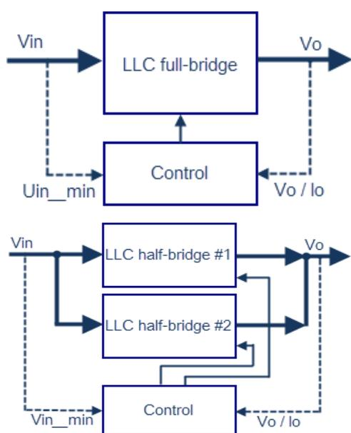
**Fig. 2.** Block schematic of full-bridge LLC converter (left) and dual half-bridge LLC converter (right)
