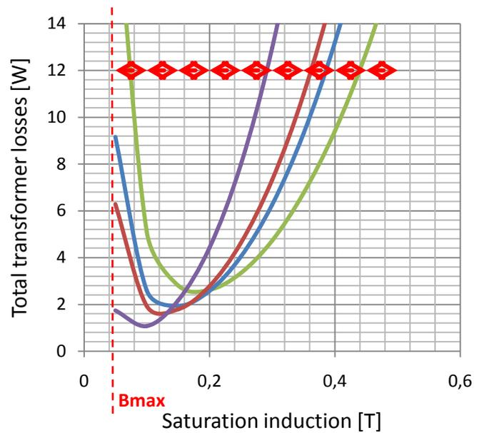
Fig. 6 Total transformer losses in dependency on the value of saturation induction and core volume
