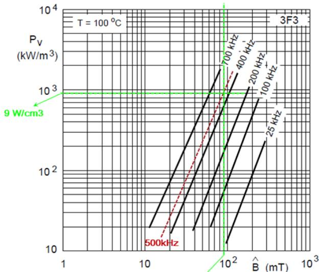
Fig. 4 Expected core losses for selected operation point
