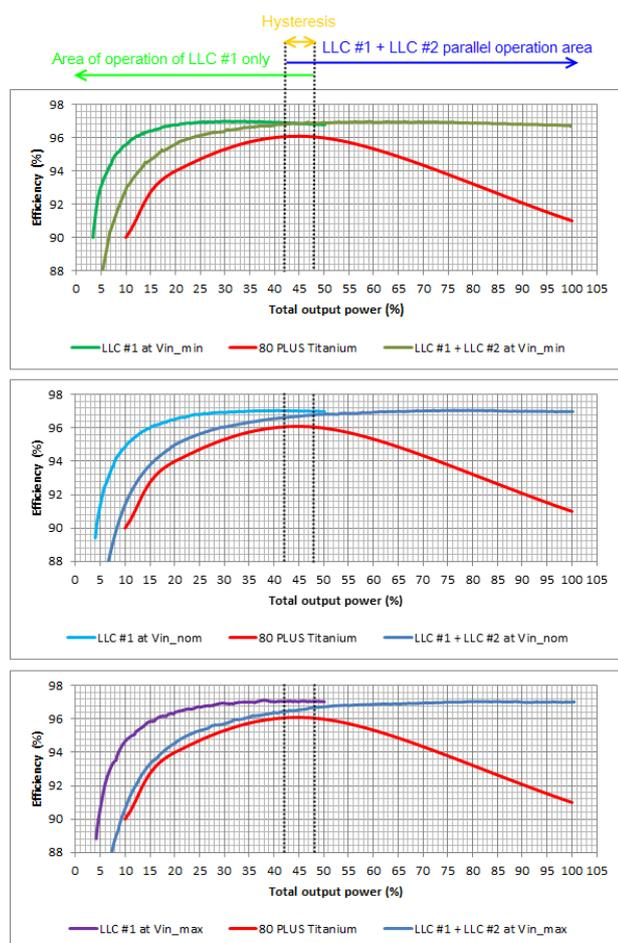
**Fig. 15** Efficiency curves of dual interleaved LLC converter received with the use of interactive control and data management
