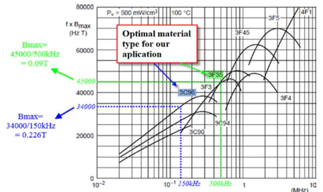
Fig. 3 Material selection curves for various operational conditions
