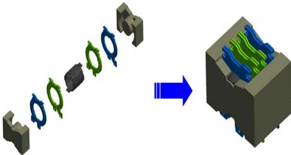
Fig. 5 Example of bobbin-less high-frequency transformer design
