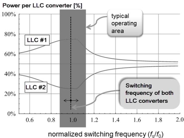
**Fig. 9** Unbalanced distribution of output power between the LLC converter due to tolerances of the resonant components
