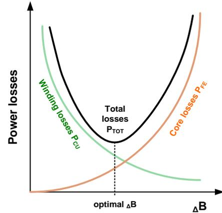
Fig. 2 Dependency of transformer losses on the ripple of magnetic induction
