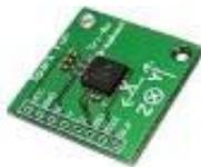
Figure 6: Accelerometer module "MMA7260Q" Freescale inc
