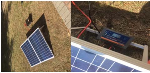
Fig. 1 shows our solar panel and charge controller delivering over 12 volts to charge our primary battery.
