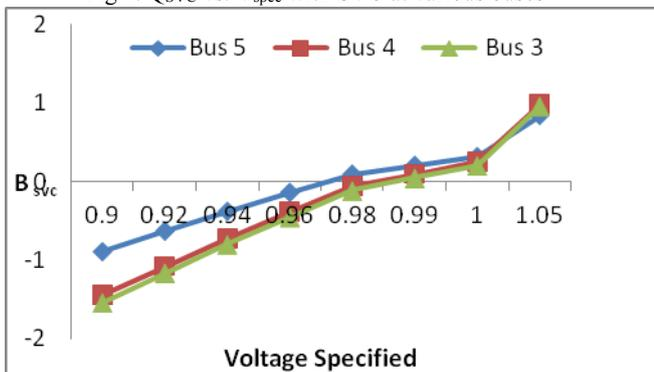
Fig 5:  $B_{svc}$  vs.  $V_{spec}$  with SVC at various buses
