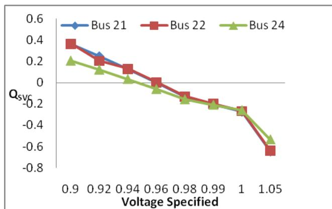
Fig 8: Variation : Q<sub>svc</sub> vs. V<sub>spec</sub> with SVC at various buses in IEEE 30 bus system
