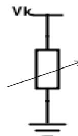
Fig 1: Static Var Compensator (Variable susceptance model)
