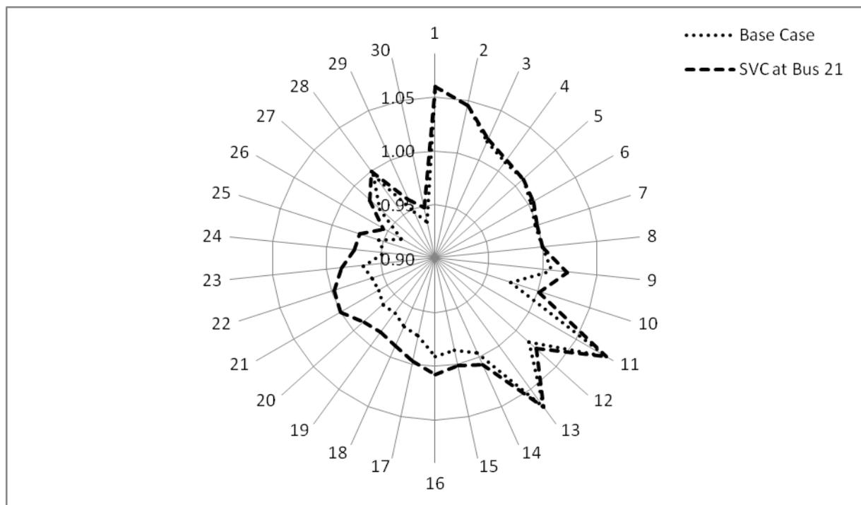
Fig 7: Comparison of voltage profile without and with SVC at bus 21
