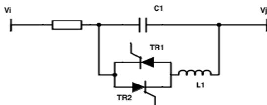
Fig 2: TCSC connected in a transmission lines between buses i and j
