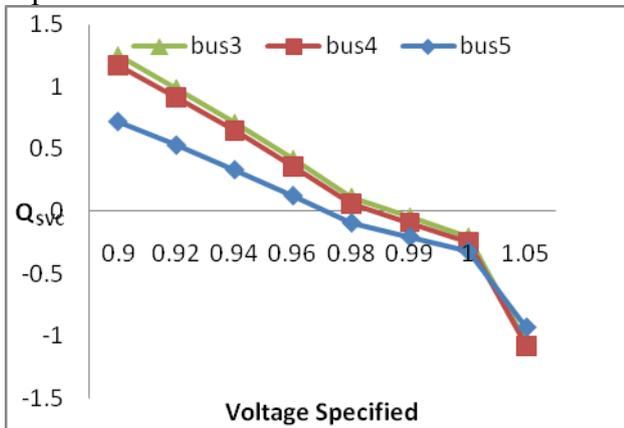
Fig 4:  $Q_{svc}$  vs.  $V_{spec}$  with SVC at various buses
