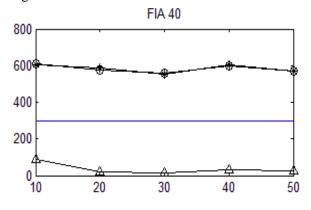
Fig 6. Variation of fault index from Bus1 at LL Fault on Phase AB for transmission line at Fault Inception Angle  $40^{\circ}$ .
