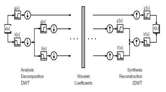
Fig 1.Analysis of signal using wavelet transforms
