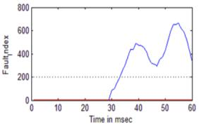
Fig 12 Detection of LG fault at PV generation
