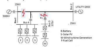
Fig 3. Single line diagram for microgrid connected to utility grid
