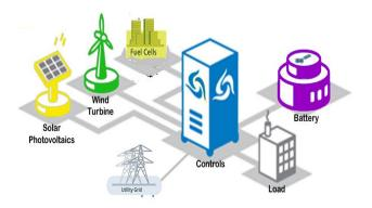
Fig 2: Microgrid connected energy resources to utility grid
