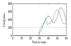
Fig 11: Detection of LLG at wind generation
