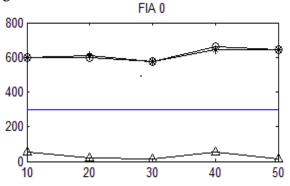
Fig 4. Variation of fault index from Bus1 at LL Fault on Phase AB for transmission line at Fault Inception Angle  $0^0$
