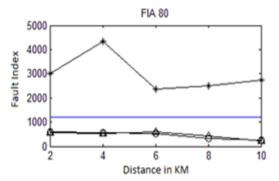
Fig7. Variation of fault index from Bus2 at LG Fault on Phase AG for transmission line at Fault Inception Angle 80<sup>0</sup>.
