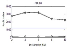
Fig8. Variation of fault index from Bus2 at LLG Fault on Phase ABCG for transmission line at Fault Inception Angle  $80^{\circ}$ .
