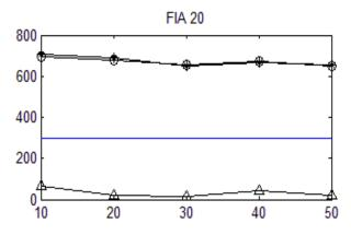
Fig 5.Variation of fault index from Bus1 at LL Fault on Phase AB for transmission line at Fault Inception Angle 20<sup>0</sup>.
