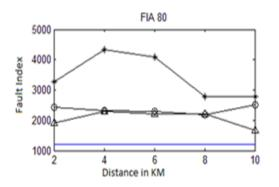
Fig9. Variation of fault index from Bus2 at LLLG Fault on Phase ABCG for transmission line at Fault Inception Angle  $80^{\circ}$ .
