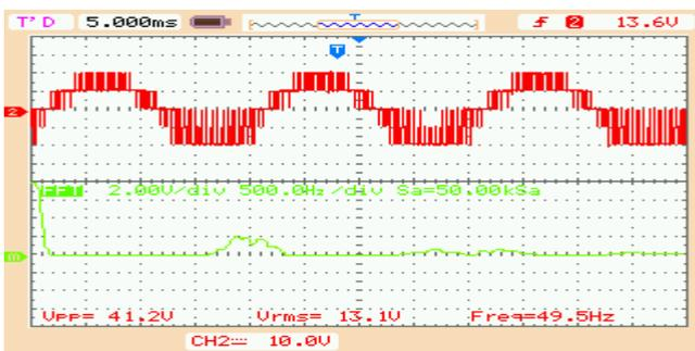
Figure. 16 Output voltage and FFT plot of cascaded MLI with (APOD+CO) PWM strategy for R-phase (sine ref.)
