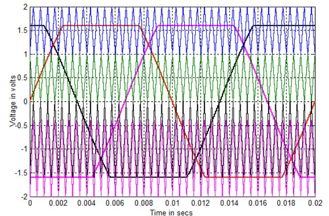
Figure. 5 Sample Carrier arrangement for (APOD + CO) hybrid PWM strategy ( $m_a = 0.8$ ,  $m_f = 40$ ) with 60 degree reference
