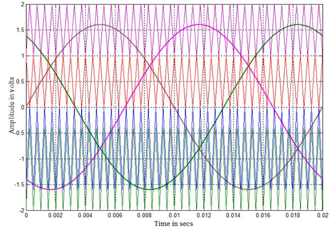
Figure. 3 Sample Carrier arrangement for (APOD + CO) hybrid PWM strategy ( $m_a = 0.8$ ,  $m_f = 40$ ) with sine reference
