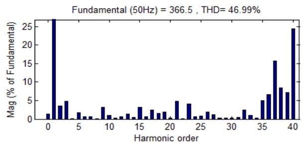
Figure. 14 FFT plot of cascaded MLI with (APOD+CO) PWM strategy for R-phase (stepped wave ref.)
