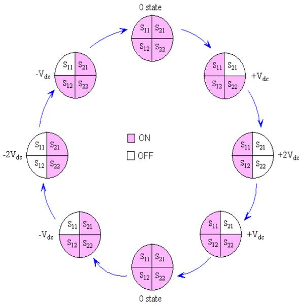
Figure. 2 Cyclic switching sequence of chosen MSMI
