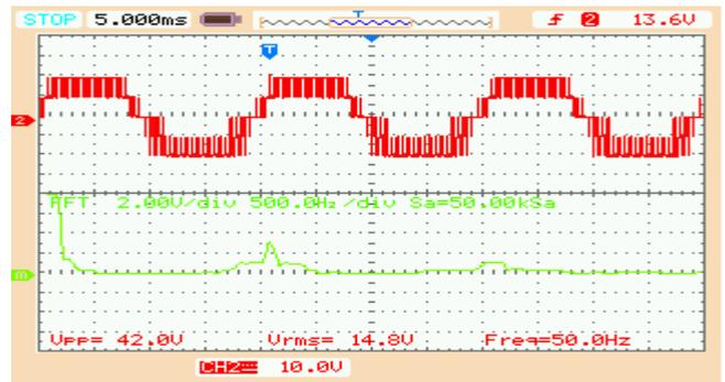
Figure. 18 Output voltage and FFT plot of cascaded MLI with (APOD+CO) PWM strategy for R-phase (60 degree ref.)
