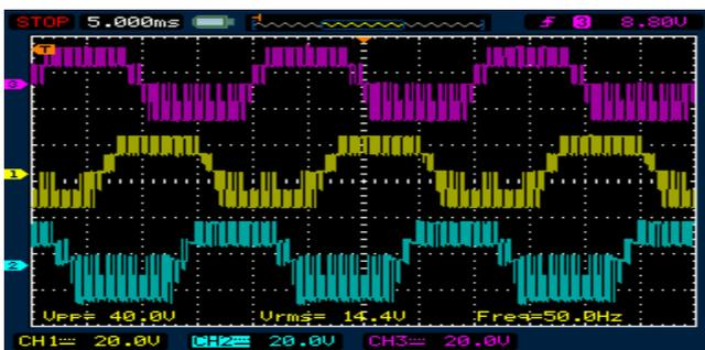
Figure. 17 Output voltage of cascaded MLI with (APOD+CO) PWM strategy (THF ref.)
