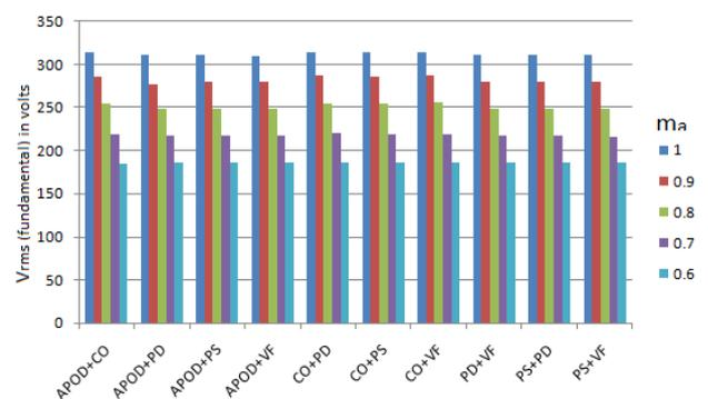
Figure. 21 Sample RMS fundamental of output voltage of cascaded MLI vs  $m_a$  with sine ref (By simulation)
