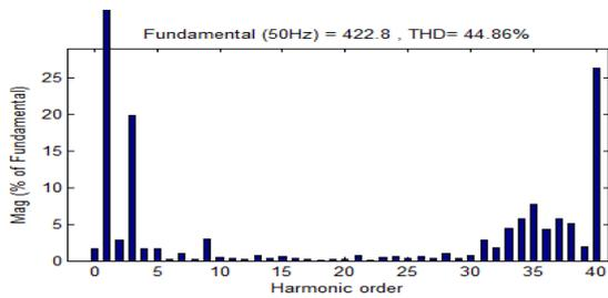
Figure. 10 FFT plot of cascaded MLI with (APOD+CO) PWM strategy for R-phase (TH1 ref.)
