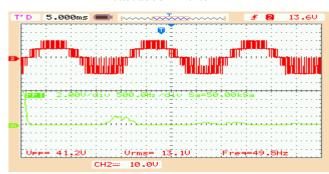
Figure. 16 Output voltage and FFT plot of cascaded MLI with (APOD+CO) PWM strategy for R-phase (sine ref.)
