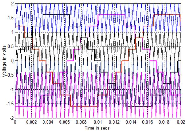
Figure. 6 Sample Carrier arrangement for (APOD + CO) hybrid PWM strategy ( $m_a = 0.8$ ,  $m_f = 40$ ) with stepped wave reference
