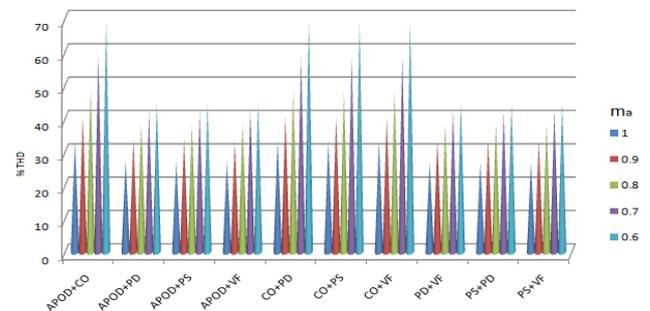
Figure. 20 Sample % THD of output voltage of cascaded MLI vs  $m_a$  with sine ref (By simulation)
