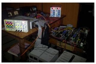
Figure. 15 Hardware setup of three phase five level cascaded inverter
