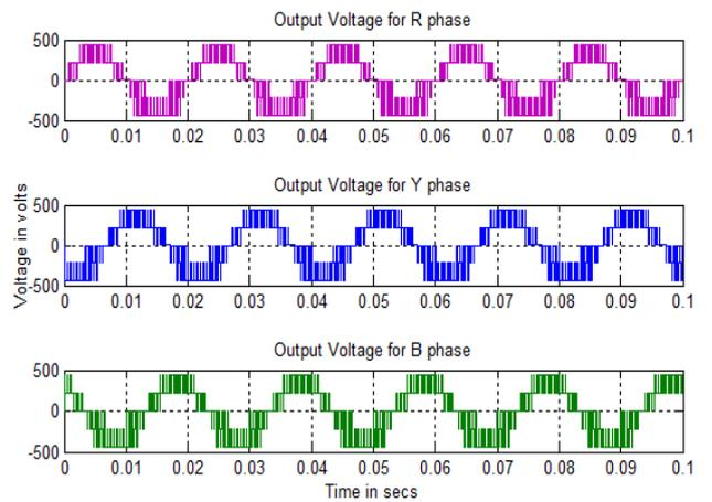
Figure. 13 Output voltage of cascaded MLI with (APOD+CO) PWM strategy (stepped wave ref.)
