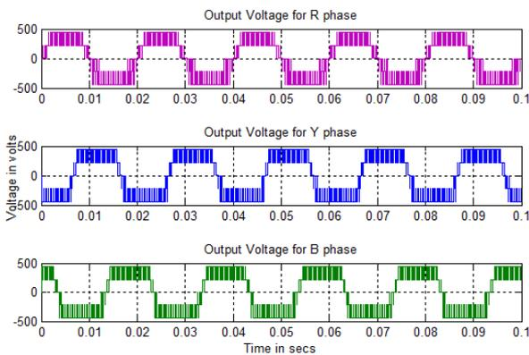
Figure. 11 Output voltage of cascaded MLI with (APOD+CO) PWM strategy (60 degree PWM ref.)
