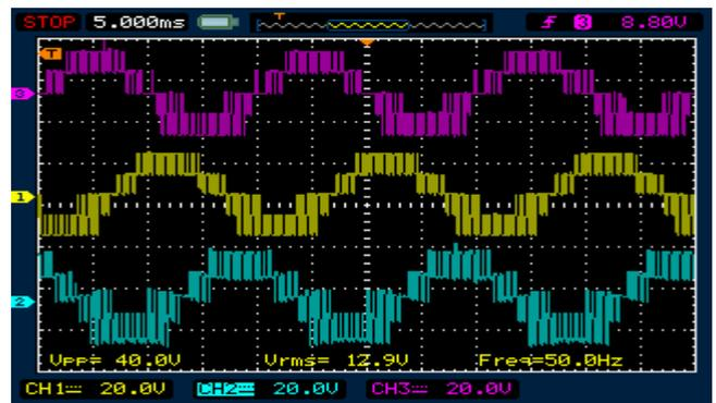
Figure. 19 Output voltage of cascaded MLI with (APOD+CO) PWM strategy (stepped wave ref.)
