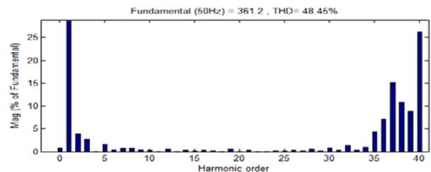
Figure. 8 FFT plot of cascaded MLI with (APOD+CO) PWM strategy for R-phase (sine ref.)
