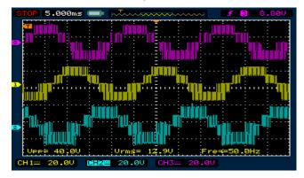
Figure. 19 Output voltage of cascaded MLI with (APOD+CO) PWM strategy (stepped wave ref.)
