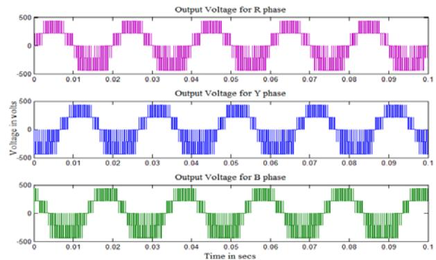
Figure. 7 Output voltage of cascaded MLI with (APOD+CO) PWM strategy (sine ref.)
