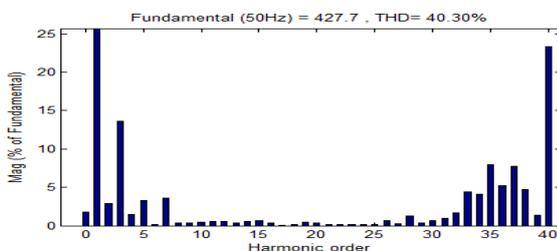
Figure. 12 FFT plot of cascaded MLI with (APOD+CO) PWM strategy for R-phase (60 degree PWM ref.)
