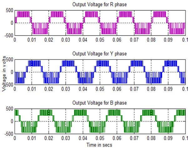
Figure. 9 Output voltage of cascaded MLI with (APOD+CO) PWM strategy (TH1 ref.)
