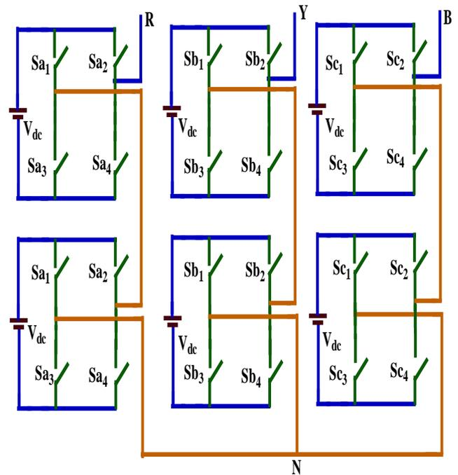
Figure. 1 Three phase five level cascaded inverter
