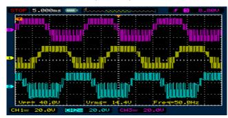
Figure. 17 Output voltage of cascaded MLI with (APOD+CO) PWM strategy (THI ref.)
