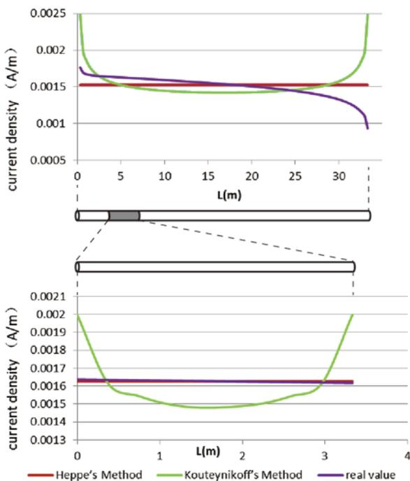
Fig. 7 Different Methods for Handling the Current Density of Segment A
