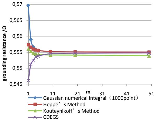
Fig. 4. Grounding Resistance Curve with Different  $m$  Based on Four Methods
