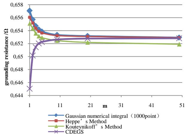
Fig. 6. Grounding Resistance Curve with Increase of  $m$  Based on Four Methods
