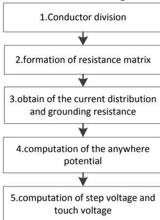
Fig. 1. Calculation Process of Equal-potential Grounding Model
