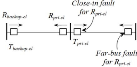
Fig. 1. Close-in and far-bus faults for primary relay.
