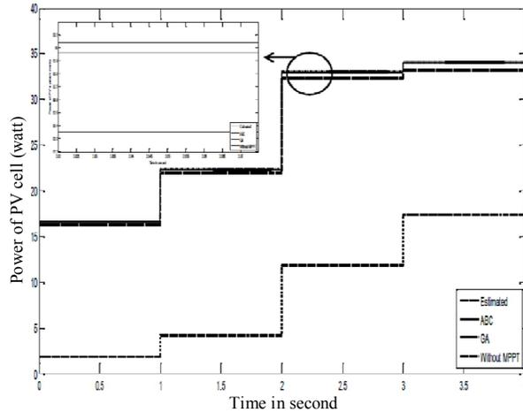
Fig. 15. Power of PV cell for different radiation and temperature.
