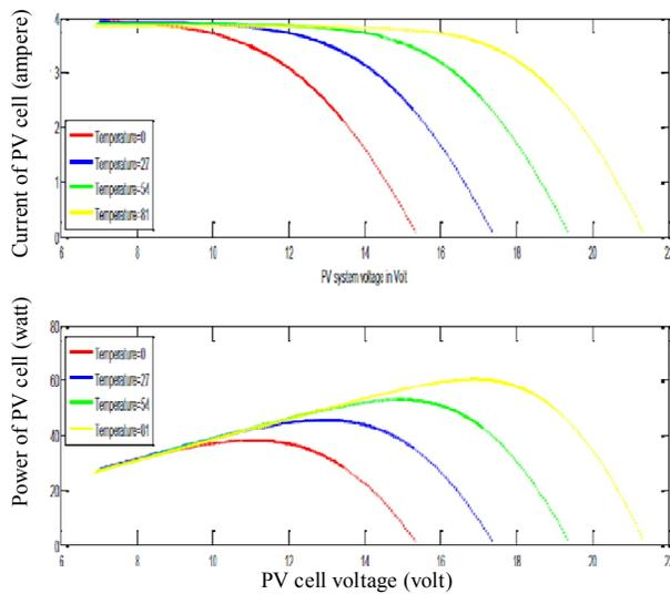
Fig. 10. Change of PV parameters with different temperature.
