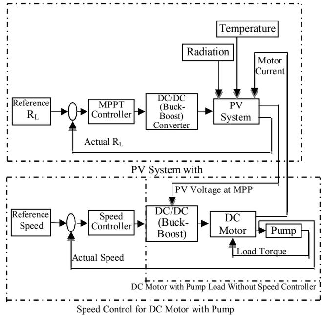
Fig. 1. Overall block diagram of DC control system supplied by PV system at MPPT.
