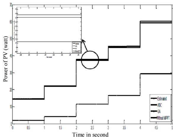
Fig. 7. Power of PV cell for different controllers.
