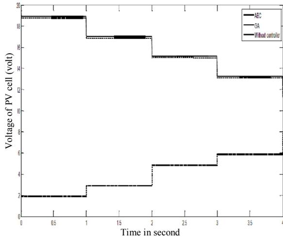
Fig. 16. Change of PV cell voltage for different radiation and temperature.
