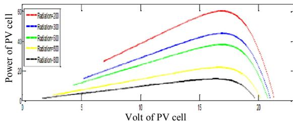
Fig. 6. Relation between volt, current, and power for different radiation.
