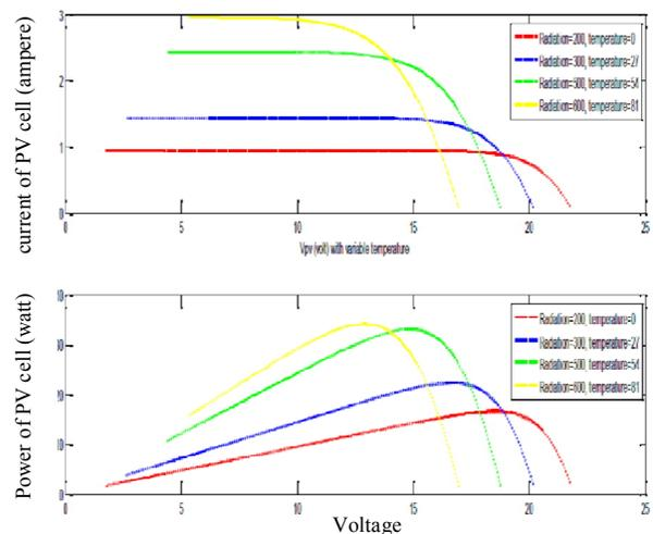
Fig. 14. Change of PV cell parameters with different radiation and temperature.
