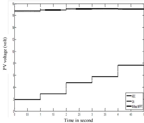
Fig. 8. Voltage of PV cell for different controllers.
