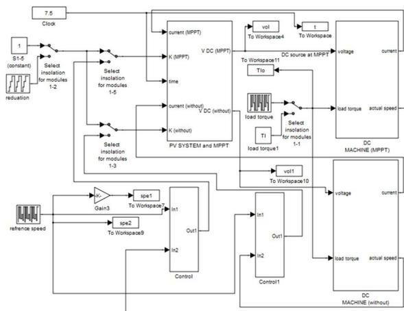
Fig. 2. Overall Matlab system of DC control system supplied by PV system at MPPT.
