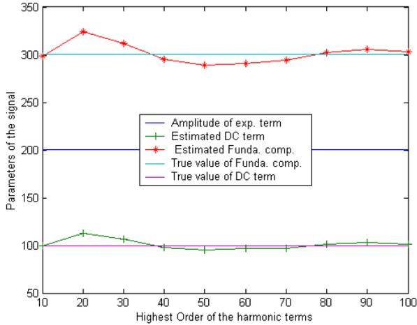
Fig. 2. Estimated parameters of the signal  $z(k)$  using proposed algorithm as a function of the order of the harmonics  $N_0$ .
