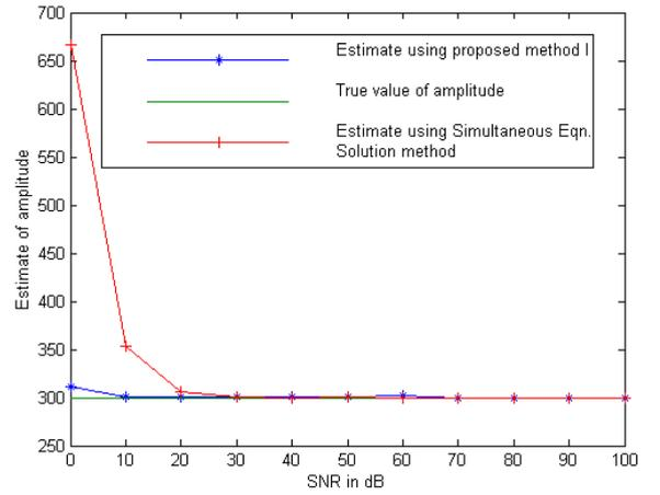
Fig. 3. Estimated amplitude of the fundamental component of the signal  $z(k)$  using the proposed algorithm in section II and simultaneous equation solution method as a function of SNR in dB for  $N_0 = 4$ .
