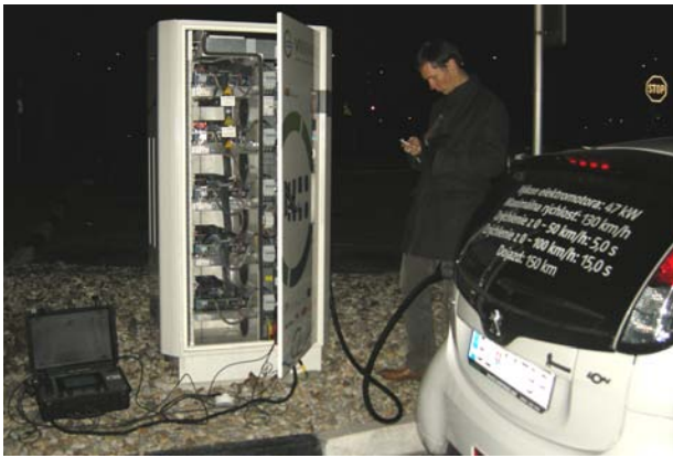
Fig. 7 Fast charger connected to electric vehicle during measuring
