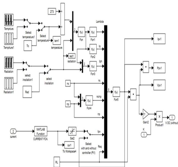
Fig. 2. Matlab/Simulink for PV system and DC-DC converter
